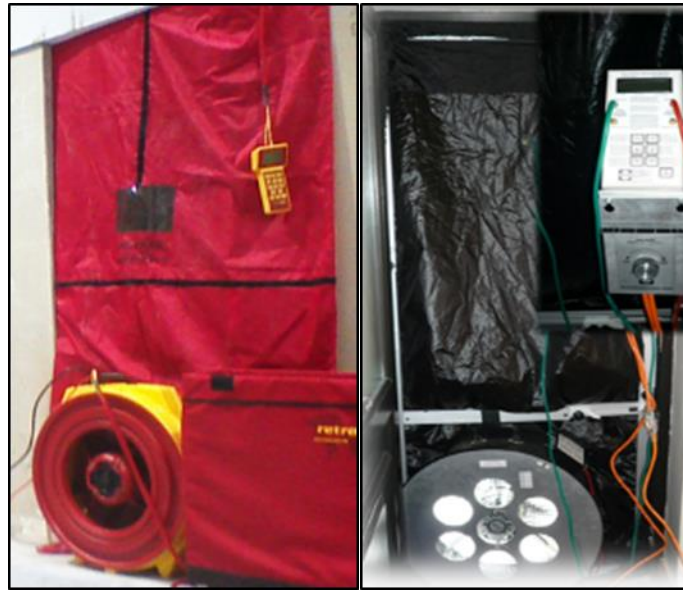
Figure 3.26 Air permeability unit with fan and monitoring equipment
